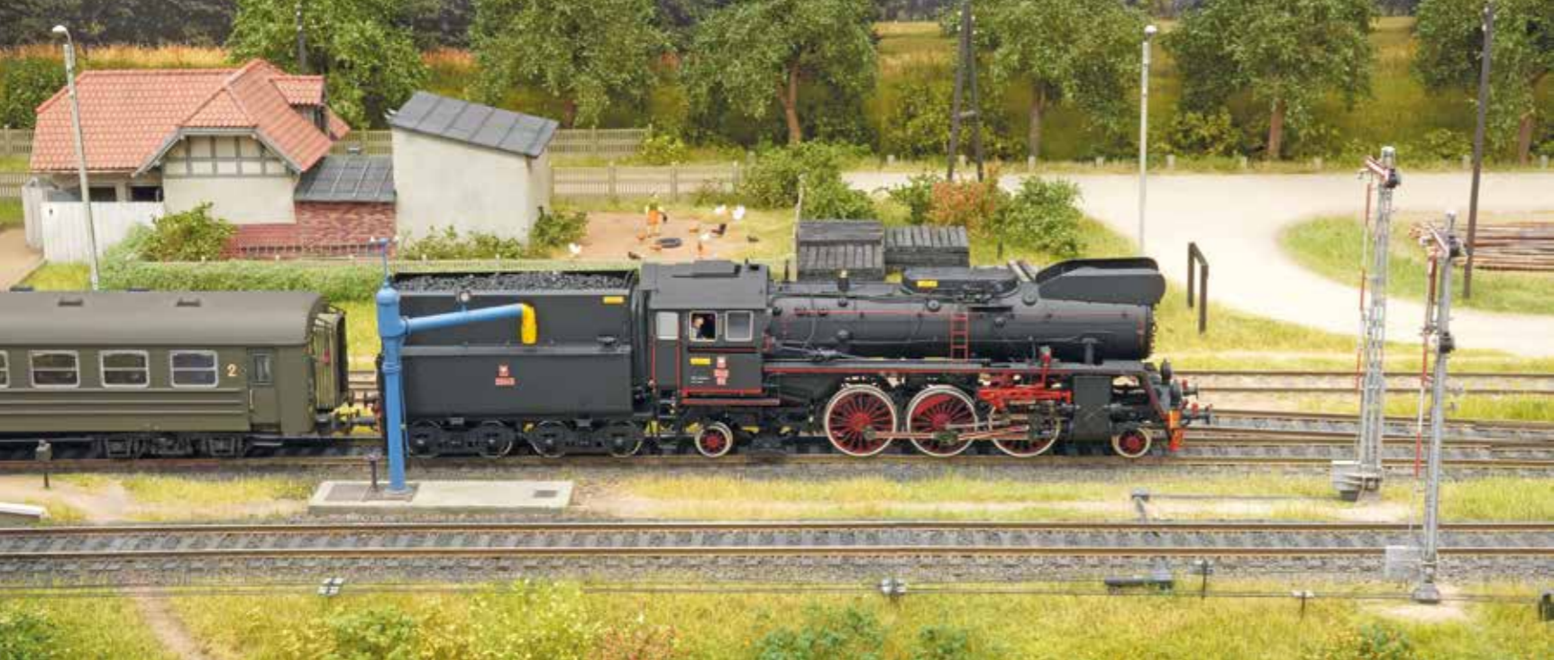
Above There are two water cranes at Wysoka Gorzowska, fed from the water tower. The models are by Auhagen but had to be 'supercharged' – the upper part can swivel operated by a servo drive switched at the control panel.
