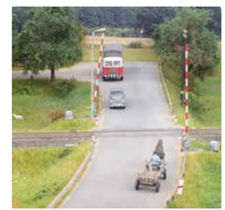
Below right The level crossing barriers were also made from Weinert Modellbau parts, with an electric drive and integrated sound module which accompanies the movement of the barriers with a bell. Immediately to the right of the crossing is the JEG-10 barrier drive with mechanical transmission via belts. The model, an exact replica of the original, is a well-designed dummy. Photos: editor.
