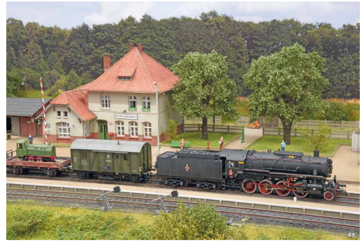
Below A goods train crew van is coupled behind the Tr-203 2-8-0. This accommodated the guard and often also a shunter.
