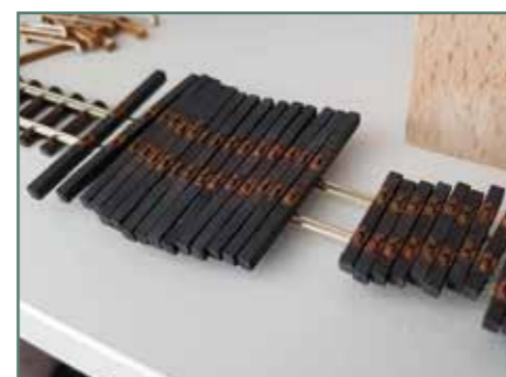
Above Special long sleepers had to be made for the bridge deck to replace the Roco originals.
